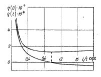
Fig. 2. Heat influx (q, W) at cold and hot ends of the lead as a function of the length chosen for it.
