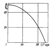
Fig. 1. Temperature distribution over length of lead.
